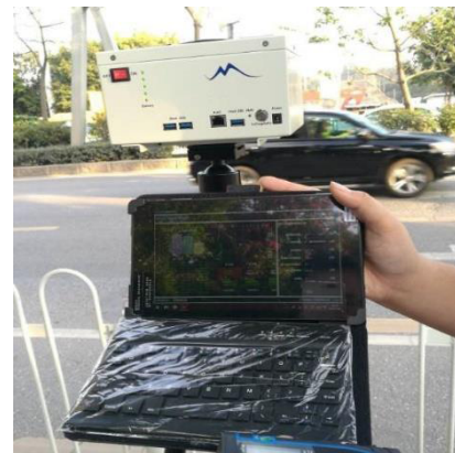
FIGURE 3. Data acquisition equipment WM-LDS3.0 portable laser survey system.
