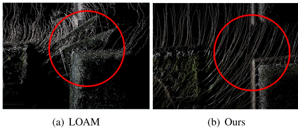
FIGURE 10. (a) The LOAM failed when passing the corner (the point cloud is colored). (b) Our approach has almost no drift in the same corner, which proves that fusing image information improves the odometry robustness.
