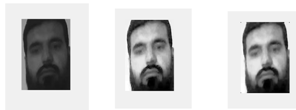
FIGURE 5. RGB scale to grayscale image, histogram equalization of image, and median filter applied to the image (left to right).
