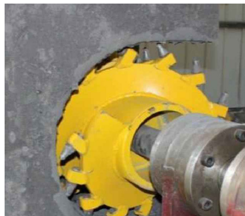
FIGURE 14. Shearer mining artificial coal wall.
