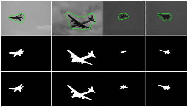
FIGURE 9. Comparison of segmentation results between our method and CRF-RNN model. The first row is the test images superimposed with initial contours, and the second to third rows are the segmentation results of the CRF-RNN and our EO-DRLSE models respectively. The relevant task parameters: \mu = 0.07 , \Delta t = 4.5 , \sigma = 4.5 and \varepsilon = 3.5 .
