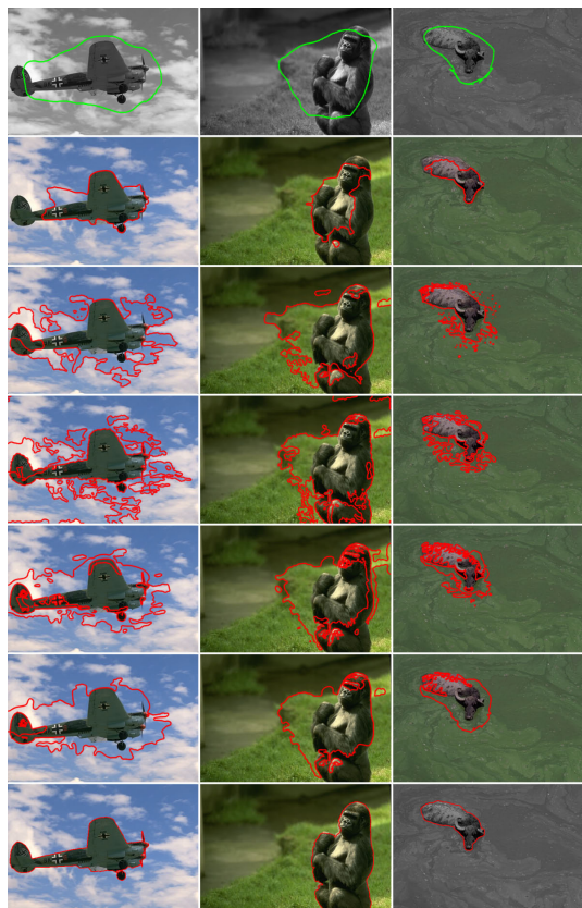
FIGURE 7. A set of comparison experiments for the robustness to the imaging noise of real-life images. The first row is the input images containing initial contours. The second to seventh rows are the segmentation results by using the DRLSE, LGDF, LIF, LPFE, RSF-LoG and our EO-DRLSE models respectively. The relevant task parameters: \mu = 0.07 , \Delta t = 4.5 , \sigma = 5.5 and \epsilon = 3.5 .
