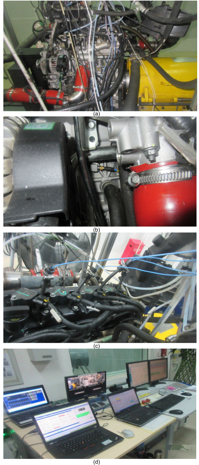
FIGURE 1. Bench test. (a) Engine. (b) Vibration sensors. (c) Cylinder pressure sensors. (d) Testing system.
