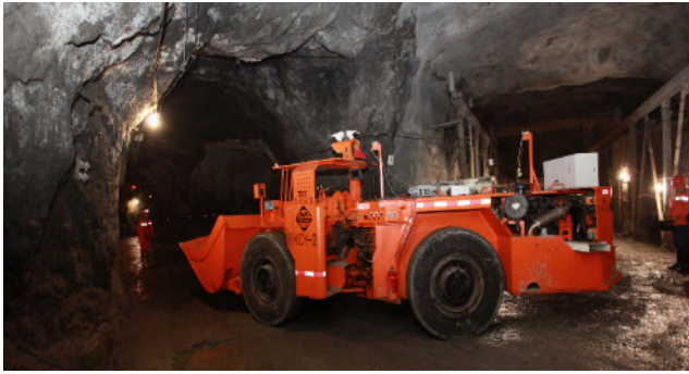
FIGURE 1. Load Haul Dump (LHD).
