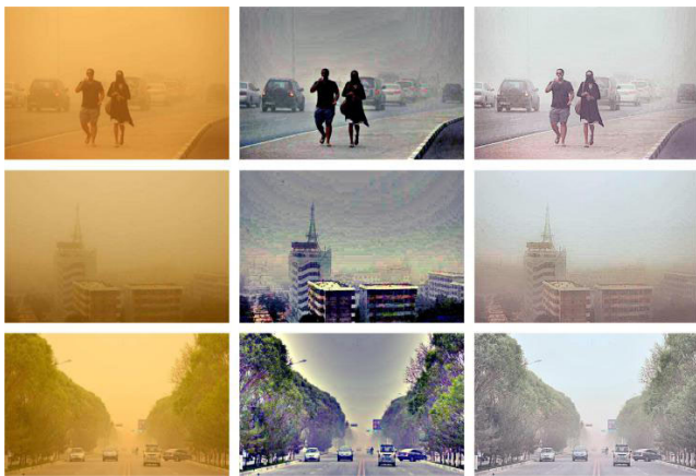
FIGURE 7. Comparisons of our method with the MSRCR [30]. left column: Sand dust images, middle column: MSRCR [30], and right column: Results using our method.
