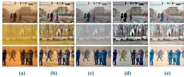
FIGURE 11. Comparisons of our method with several state-of-the-art sand dust image enhancement methods. (a) Synthesized sand dust images, (b) results using CLAHE, (c) results using Wang's method, (d) results using the MSRCR, and (e) results using our method.
