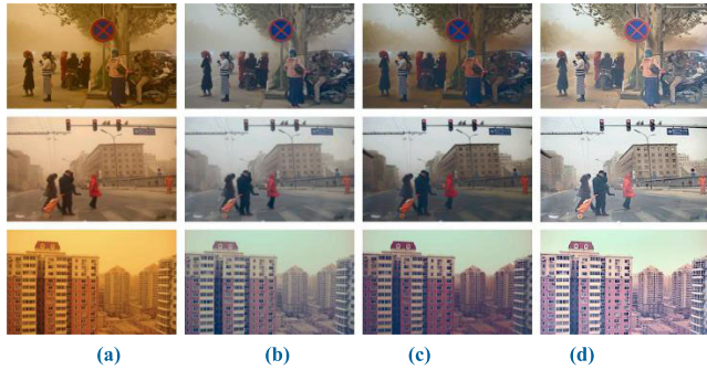
FIGURE 3. Illustration of sand dust image enhancement results using our proposed method. (a) Input sand dust image, (b) color recovered images, (c) dust haze removed images, and (d) final output images with our method.
