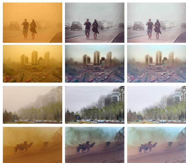
FIGURE 14. Comparisons of our proposed NGC improved CLAHE with the original CLAHE. left column: Sand dust images, middle column: illumination adjustment results using the original CLAHE, right column: illumination adjustment results using our NGC improved CLAHE.
