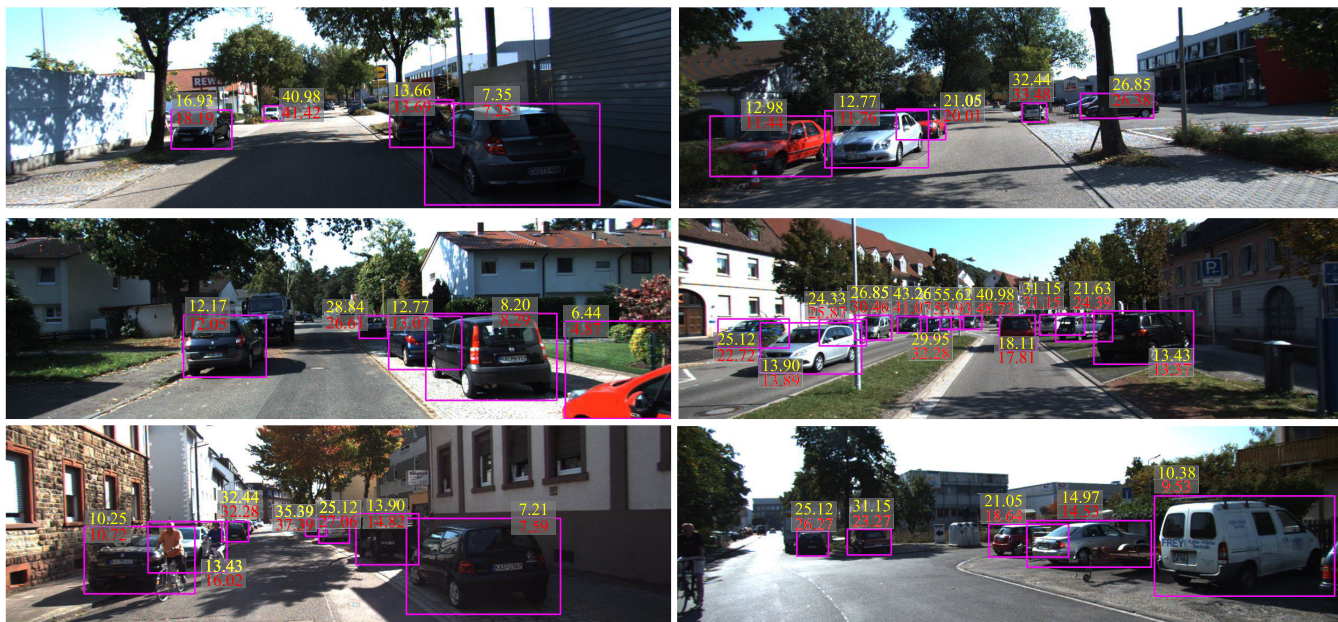
FIGURE 9. Examples of object-level depth estimation results on KITTI evaluation set using Disparity Detector (with anchor pair ). The number in bold-red is the ground-truth depth, and the number in bold-yellow is the predicted depth from our method.
