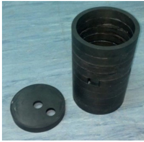
FIGURE 8. Cylindrical ferrite shields made of PC40 ferrite annuli.
