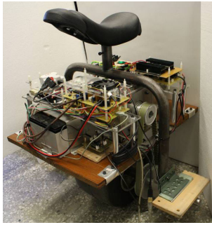
FIGURE 2. Single-wheel transportation vehicle.
