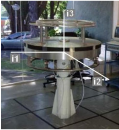
FIGURE 8. Air bearing table for satellite attitude control. Reprinted from: [39].
