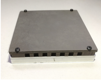
FIGURE 7. Overall view of the assembled 10 × 10 single-polarized TCDA.
