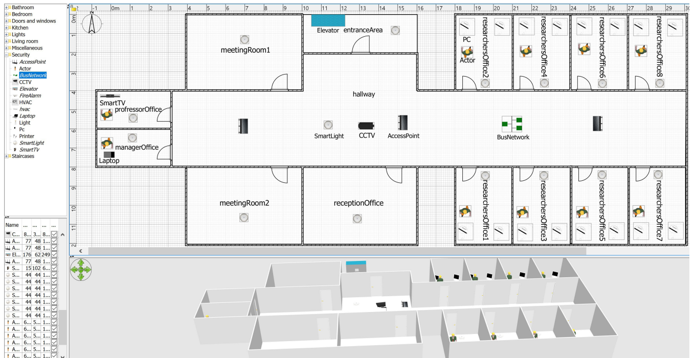
FIGURE 18. A model of the research center floor that we created using the System editor .
