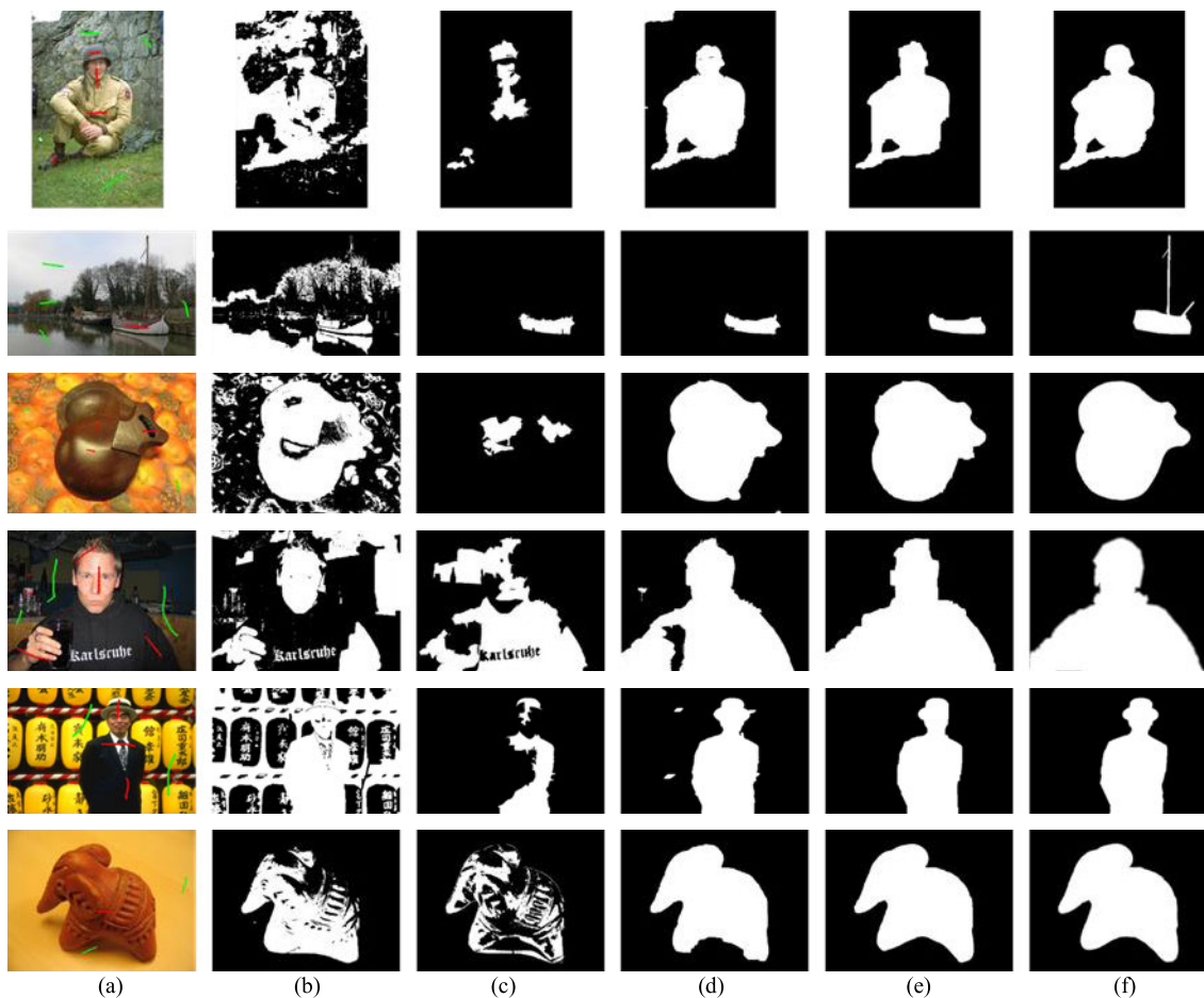
FIGURE 7. Segmentations with a few scribbles: (a) Input images with scribbles, (b) One Cut, (c) GBMR, (d) NHO, (e) Ours, and (f) ground truth.
