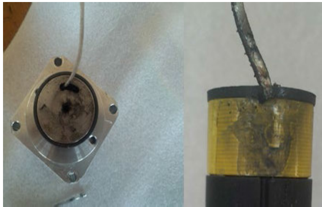
FIGURE 7. The picture of actuator coil wiring after running 300 hours.
