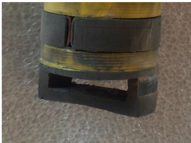
FIGURE 8. The picture of actuator skeleton after running 300 hours.
