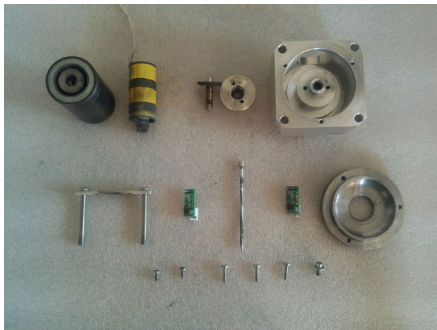
FIGURE 13. The disassembly picture of ELA after running 300 hours.
