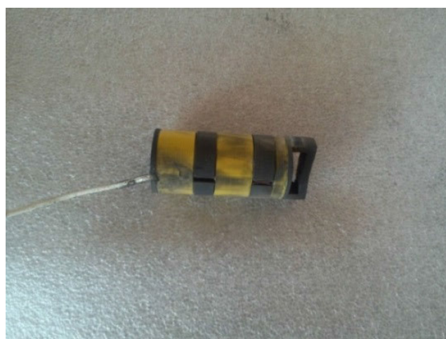
FIGURE 6. The picture of actuator coil's enameled wire abrasion after running 300 hours.
