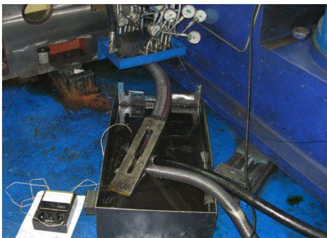
FIGURE 12. Measuring device of return oil temperature.
