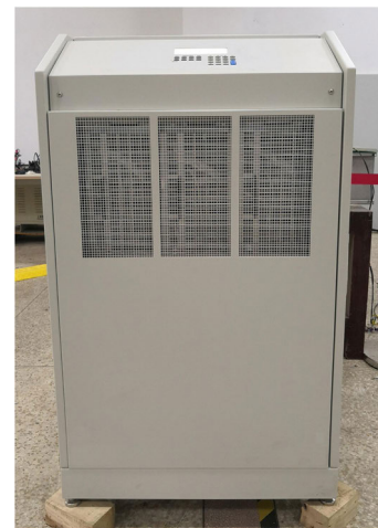
FIGURE 12. The programmable power supply device.
