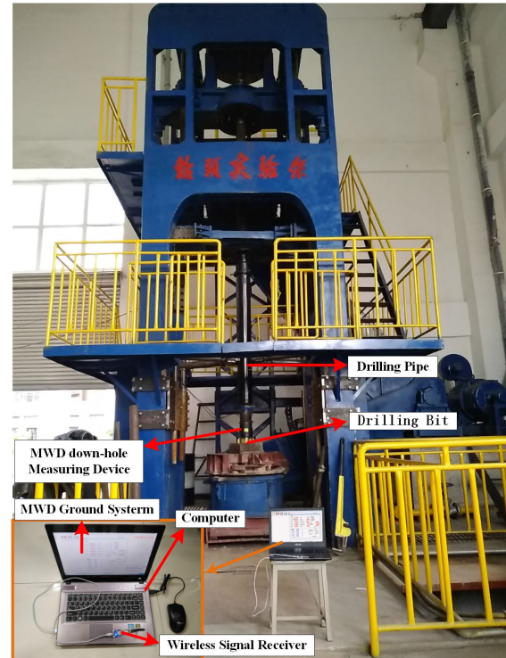
FIGURE 5. Experimental scene of measuring while drilling.
