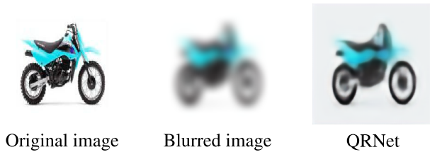
FIGURE 1. Quality recovered image from the blurred image. Original image (left), blurred image (center), quality recovered image (right). The quality recovered image was reconstructed using the proposed network, QRNet.
