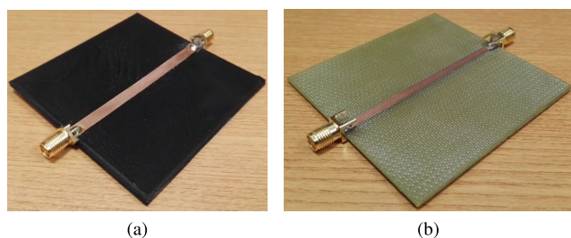
FIGURE 6. Constructed microstrip lines. a) 3D-Printed substrate with copper foil. b) FR-4 substrate with etched copper line.
