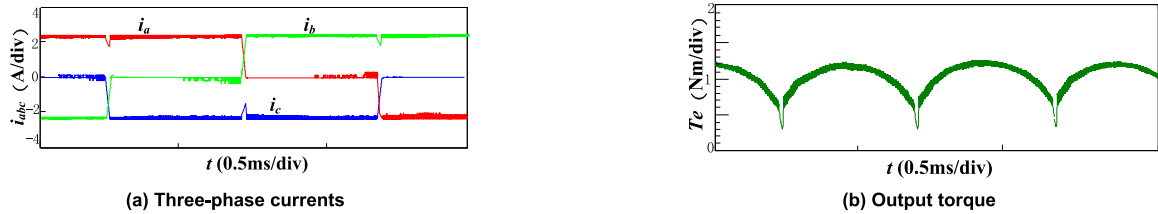
FIGURE 11. Simulation waveforms of BLDCM with the current-loop control method in PWM-ON pattern.
