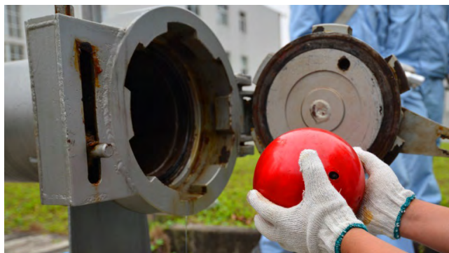
FIGURE 3. PISD rolling acceleration test in the pipeline.
