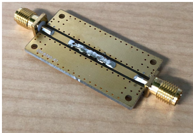
FIGURE 6. Photograph of the GCPW thru-connection board. The dimensions and materials are the same as used on the designed phone board.
