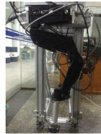
(b) Leg hydraulic drive system
