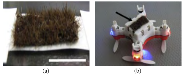
FIGURE 14. (a) Vertically aligned animal hairs on a tape with an ILG coating; (b) ILG-coated animal-hair-modified artificial pollinator [90].
