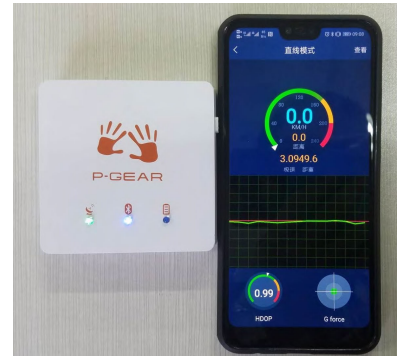
FIGURE 19. P-Gear P-510 professional satellite speed meter.
