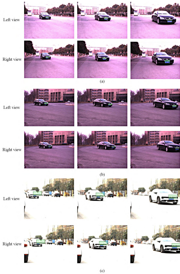
FIGURE 20. Single vehicle speed measurement experiments. (a) Straight line motion with a constant speed. (b) Curved motion with a constant speed. (c) Straight line motion with a changing speed.
