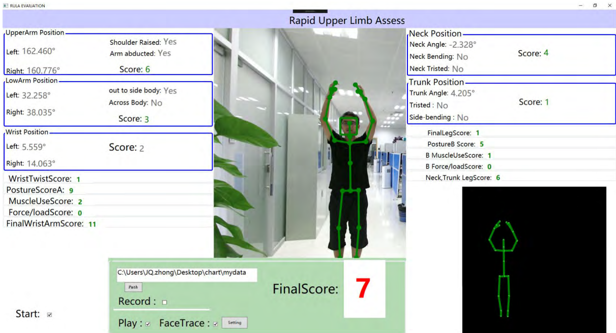
FIGURE 10. Overview of RULA GUI based on Kinect v2. It can automatically capture the assessment parameters and give RULA score in real time. Most of the parameters are from RULA worksheet of Fig. 18. Fig. 11 shows the calculation of neck side bending, trunk side-bending and trunk twist.
