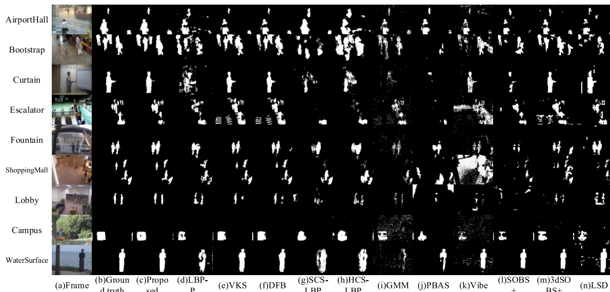
FIGURE 6. The results of 9 videos from the I2R dataset. Column (a) is the truth, (b) is groundtruth, (c) is the proposed method, and others are traditional algorithms.
