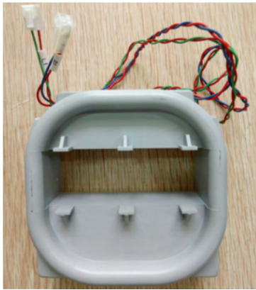
FIGURE 5. The current transformer.
