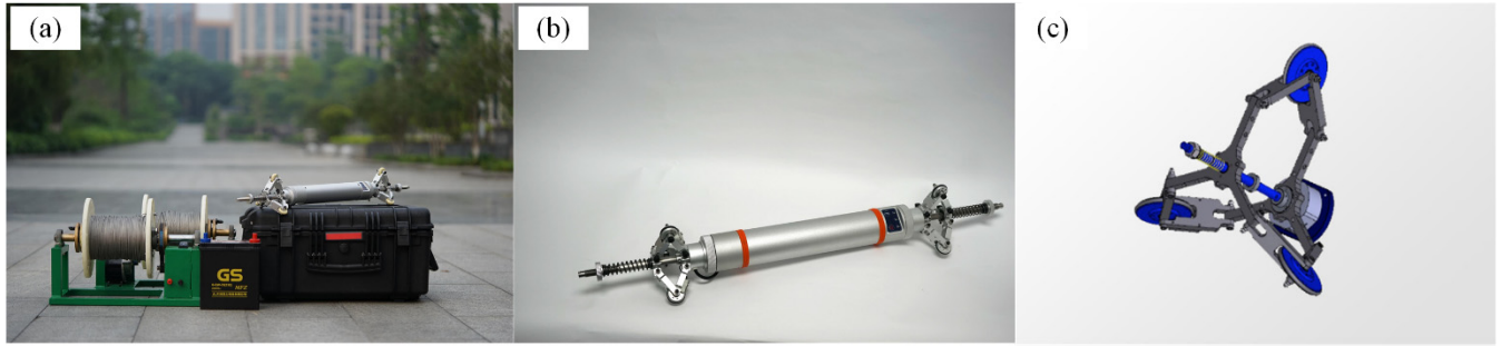
FIGURE 1. The pipeline surveying apparatus based on the MEMS IMU and odometers. (a) PIG suites, (b) PIG, and (c) self-adjusting wheelset.
