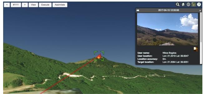
**FIGURE 6.** The *CITISENS viewer* application displays a *reference report* which targets an easily identifiable location in the photorealistic virtual world. At the top right corner, we see the corresponding view from the camera.
