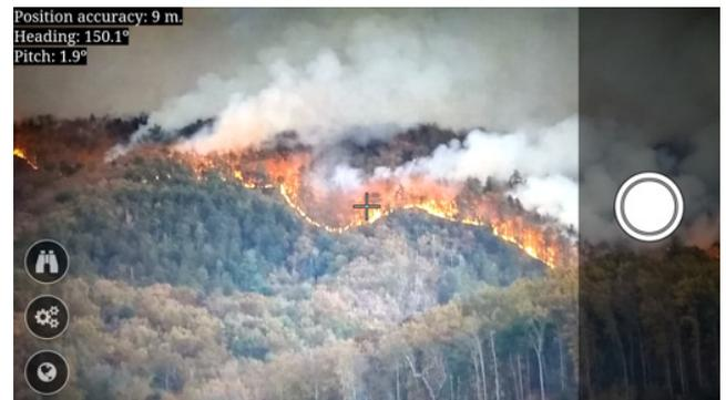
**FIGURE 2.** The user interface of the *CITISENS* reporter mobile app. The geographic coordinates of the spot behind the cross in the middle of the screen are calculated instantly once the user hits the shutter button.
