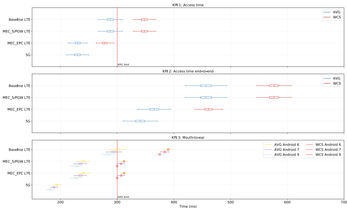
FIGURE 6. Impact of the evolution towards 5G architectures on mouth-to-ear latency.
