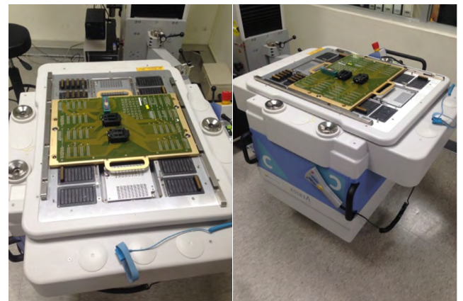
FIGURE 19. Measurement environment with ADVANTEST V93000 PS1600 automatic test system.
