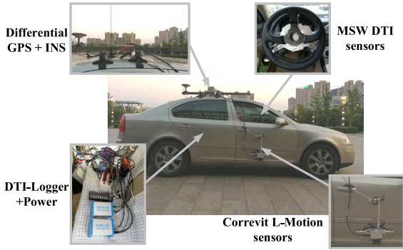
FIGURE 4. Experimental vehicle and experimental equipments.
