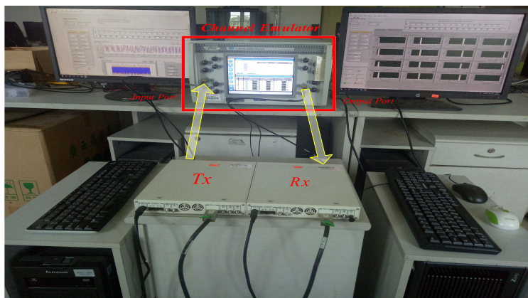
FIGURE 14. System test in doppler channel.
