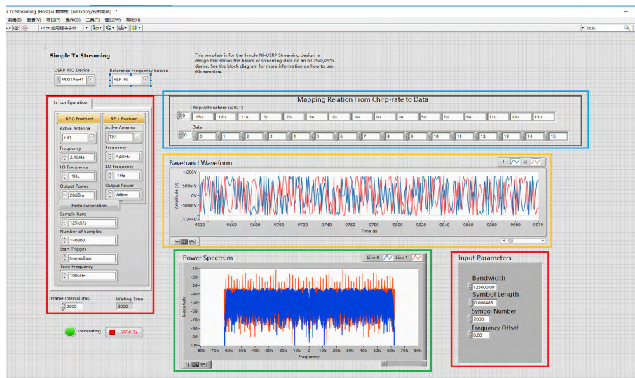
FIGURE 12. Display interface of real-time signal processing at transmitter.
