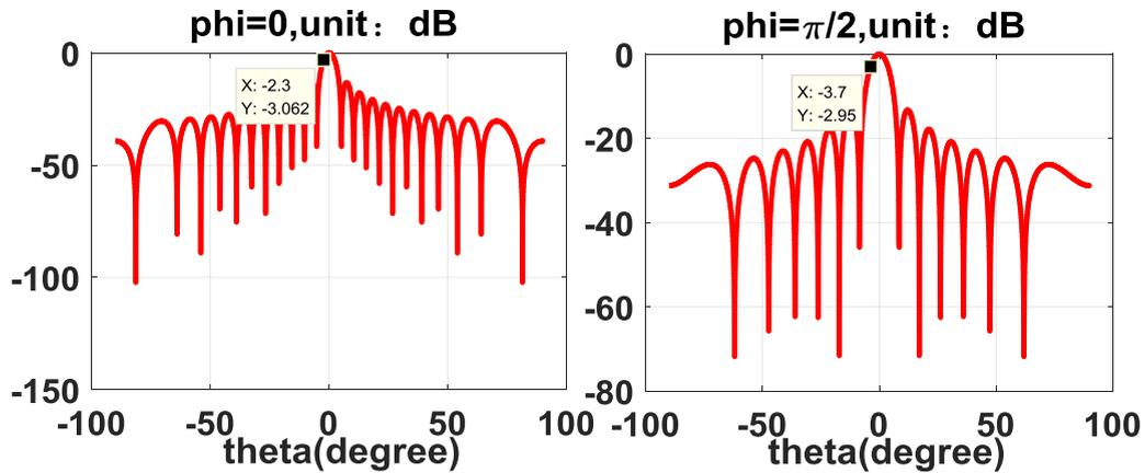
FIGURE 3. Radiation pattern of radiometer antenna.
