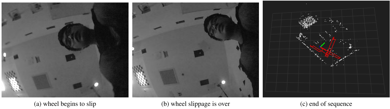
FIGURE 9. Captured images when the platform begins to experience wheel slippage and wheel slippage is over, and the finally reconstructed 3D map at the end of the sequence.
