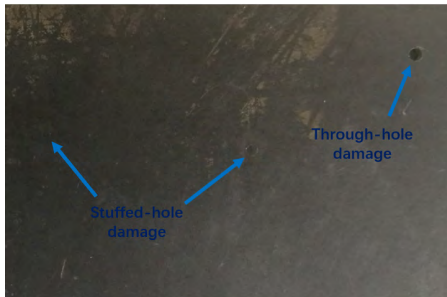
FIGURE 16. Alloy-steel plate with artificial through-hole damage and stuffed-hole damage.
