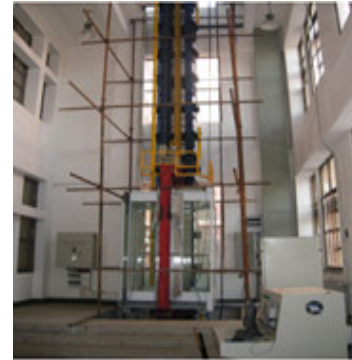
FIGURE 22. SW-PMLSM industrial hoist prototype.
