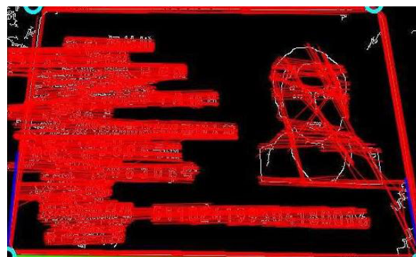
FIGURE 5. Correcting skew image by checking those lines.
