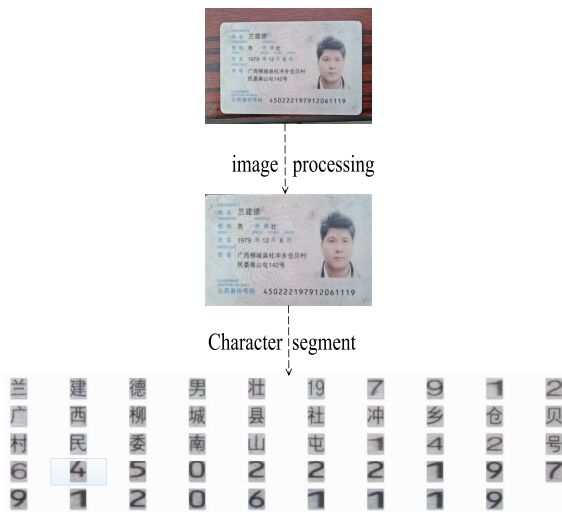
FIGURE 10. The segmentation result of an “artificial” ID card, the segmentary effect and the pieces (samples) are the real data when we train our model. The recognition accuracy has been significantly increased since these artificial samples were added into the train set.
