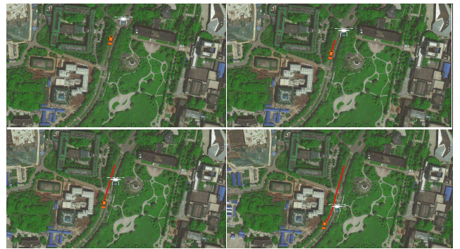
FIGURE 16. The result of geolocation at several moments. The GPS position of the target vehicle and UAV is shown on Amap. The trajectory of the target vehicle is drawn with the red line.
