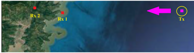
FIGURE 11. Experiment scenario. The ship-borne transmitter was located 12 m high above sea level and the receivers were installed on the land.
