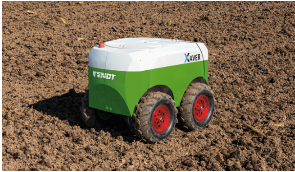
FIGURE 7. Skid-steered robot for corn seeding provided by AGCO GmbH | Fendt.
