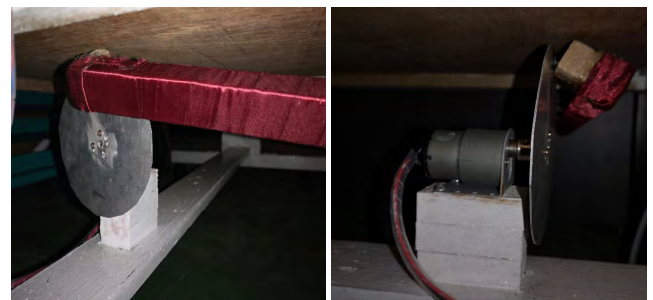
FIGURE 9. Rotating mechanism of the baby cradle.
