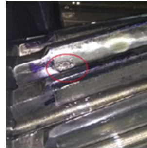
FIGURE 17. Gear with pitting fault.
