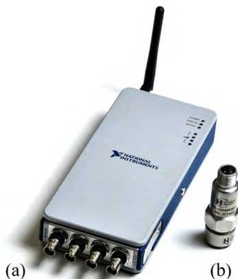
FIGURE 2. (a) National Instruments' cDAQ-9191 wireless data acquisition unit and NI-9234 sound and vibration input module. (b) Hansford sensors' HS-1005005001 IEPE accelerometer. HS-1005005001 has a magnet attached to the bottom of the sensor.
