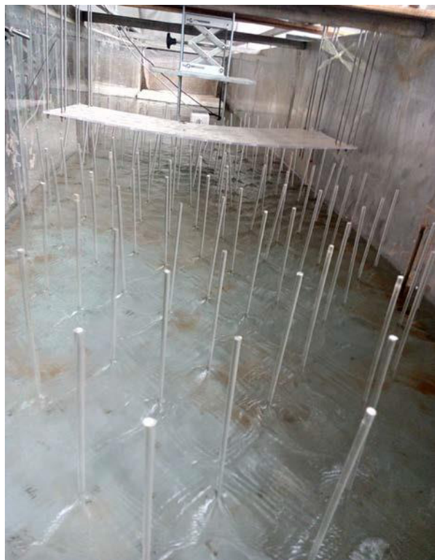
FIGURE 2. The vegetated open channel with load cell.
