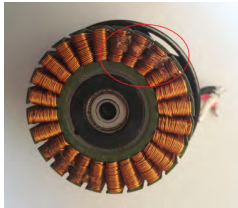
FIGURE 7. Short circuit fault of the actuator.
