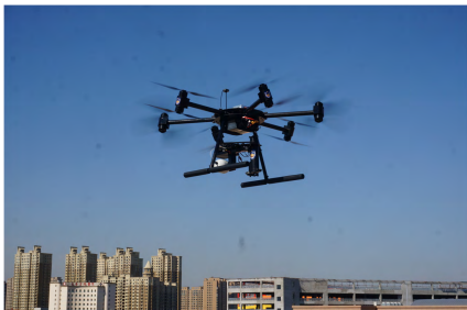
FIGURE 15. Flight experiment of Hex-Rotor UAV.
