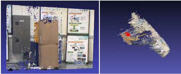
FIGURE 16. A front and top view of the fused 3D model for Cs-137 source. The model solves the visual ambiguity of overlaying 2D isotopes above vision images. Gamma source shown in red color lies behind the obstacle.
