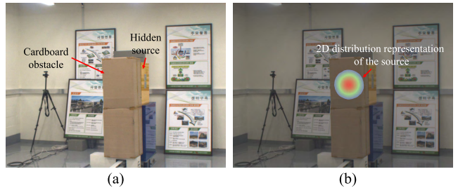
FIGURE 13. A forward representation of the Cs-137 source: (a) source is completely covered by a thick cardboard box, making it difficult to identify by the camera image, (b) an erroneous visualization of the source by overlaying isotopes above the scene image.
